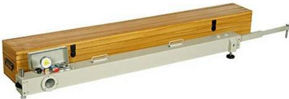
The light weight instrument is supplied in two parts for assembling on site with easy hand tools. In use one end of the beam rests at a point under investigation while the beam is pivoted at the centre. The free end carries a dial gauge to record the deflections. The other end is 2:1 which magnifies even small deflections. Supplied with a dial gauge 0.01 X 25mm. This is a light weight dismantle able instrument and easy to carry.
