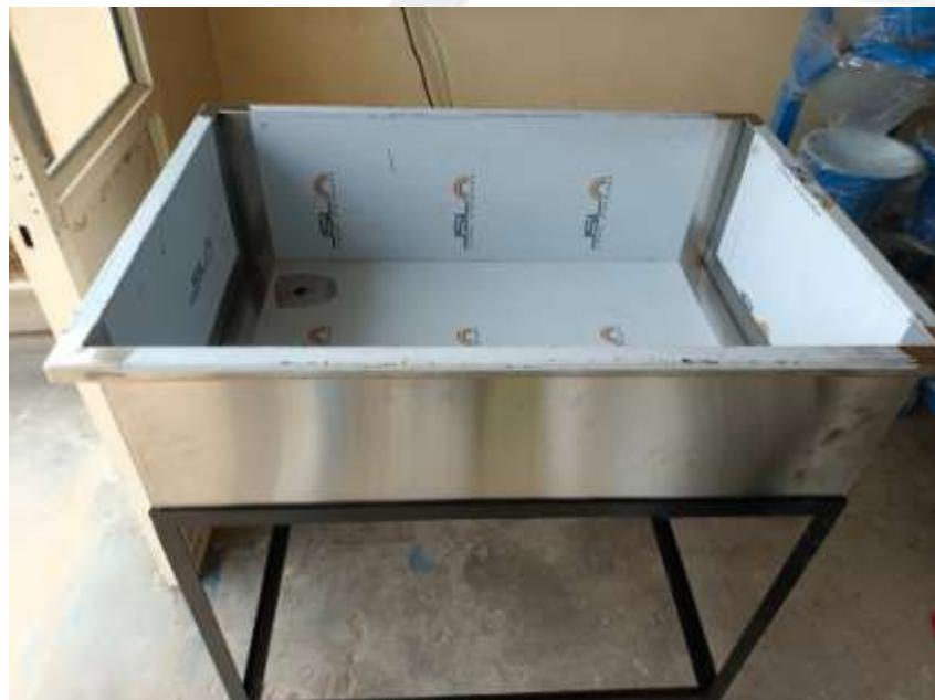
CBR Soaking Tank These tanks are made with SS 316 material and designed to suit positive tubular plate lug are hanging on supporting rib. Easy maintenance, light weighted, good chemical and weather resistant are the basic features of pickling tank which are appreciated among our clients. This is for 6 CBR moulds.
