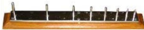
Aggregates which are flaky and/or elongated will often lower the workability of a concrete mix and may also affect long term durability. In bituminous mixtures, flaky aggregates make for a harsh mix and may also crack and break up during compacting by rolling. The flakiness of aggregates is determined by measuring the thickness of individual particles. UMI offers thickness gauge and length gauge per IS: 2386 (Part 1) to check flakiness index and elongation index of the aggregate respectively.
